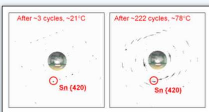
Change in microstructure of lead-free solder joints after thermal cycling. After 220 cycles the diffraction patterns develop streaks, reflecting changes in the structure of the materials used in the joint.
