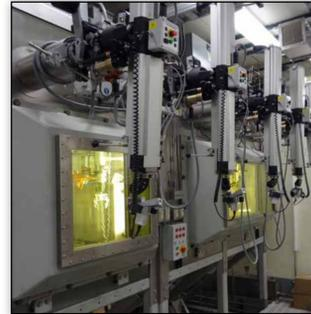
Cells for testing materials at the Advanced Test Reactor
